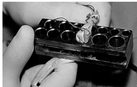
Fig. 3. The size of the knots and the smallest diameter of the loops (midportion) are measured using a template in 0.5 mm steps.
